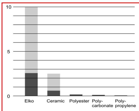
Figure 3: Dielectric absorption
