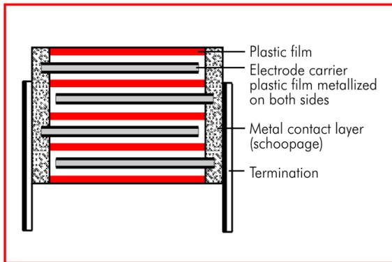
Figure 8: Cross section of WIMA MKP 10
