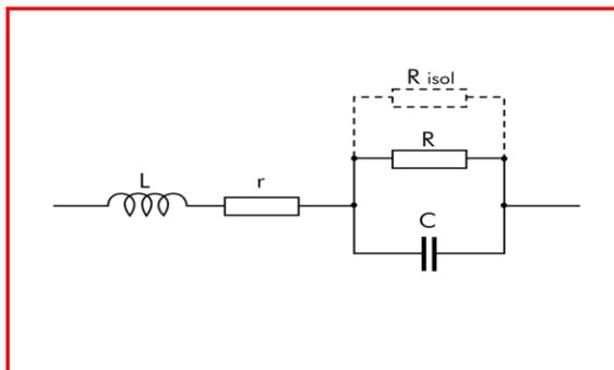
Figure 1: Equivalent circuit diagram
